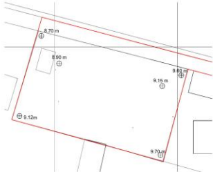
Site levels in metres Scale 1:250
